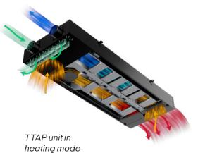
Each TTAP unit is connected to a pair of overhead ducts. The supply duct carries pre-conditioned fresh air from the AHU to each TTAP unit. The return duct carries TTAP-extracted air back to the AHU.
