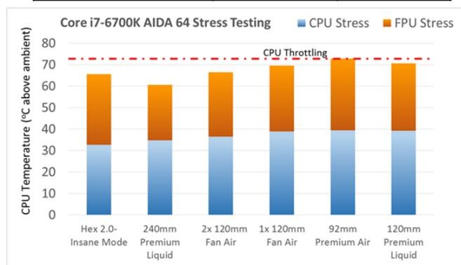
similar cooling to the much larger 2x120mm and 240mm based solutions. Only the 240mm AiO cooler was able to outperform the HEX 2.0.
